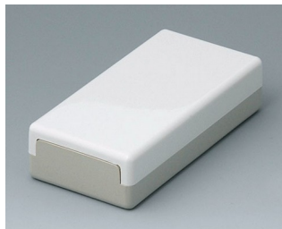
A9010065 FLAT-PACK CASE 100 N, исп. I АБС (UL 94 HB) белый RAL 9002 100x50x25mm IP 40
