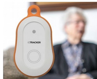
LoRa GPS tracker with alarm button
