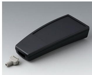
A9068129 SMART-CASE XL, исп. III АБС (UL 94 HB) черный RAL 9005 168x74,4x35,4mm IP 65 opt.
