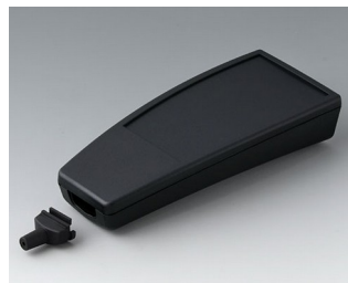
A9068349 SMART-CASE XL, исп. V АБС (UL 94 HB) черный RAL 9005 168x74,4x35,4mm IP 65 opt.
