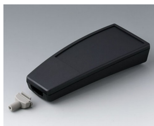
A9068149 SMART-CASE XL, исп. V АБС (UL 94 HB) черный RAL 9005 168x74,4x35,4mm IP 65 opt.
